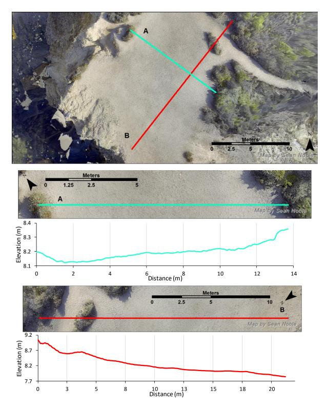
Figure 29: Cross sections of the Slot 1 bluff from the photogrammetry survey. The areas that still have vegetation were approximated 0.1 - 0.2 m higher than the adjacent devegetated areas.
