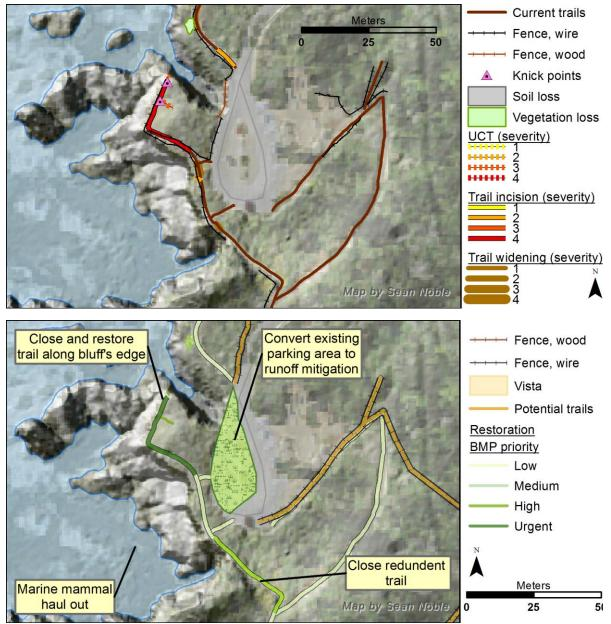
Figure 25: Suggested alternate design for the Bird Island parking area to avoid runoff into the ASBS. This would significantly reduce the amount of available parking in the area, but may be preferable to completely closing the parking lot. Significant research would have to be conducted to ensure that appropriate runoff mitigation could be implemented in the given space. Contrary to what the figure suggests using the existing ADA trail is preferable.
