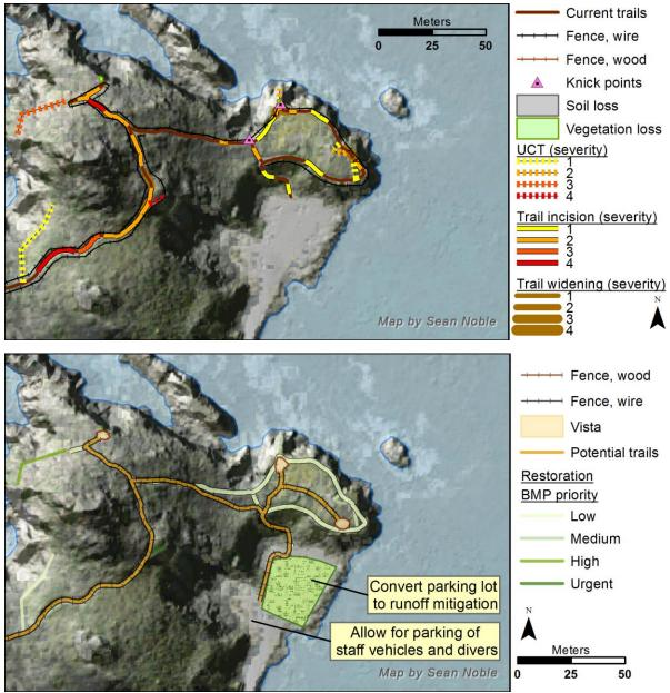
Figure 26: Suggested alternate design for the Whalers Point parking area to avoid runoff into the ASBS. Runoff down the road would have to be diverted towards the runoff mitigation. Similar to the Bird Island area, significant research would have to be done to determine what runoff mitigation could be implemented and how effective it may be.
