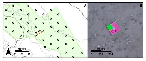
Figure 6: The planned distribution of GCP for structure through motion survey (A) and an example of one of the GCP's used (B). The spacing of the GCP's was determined through testing the viewing area from the GOPro camera from the height of the painter's pole. The multicolored pattern and numbering on the GCP's made photo identification in PhotoScan more efficient.
